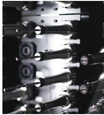
All the machines in the line are equipped with identical tool magazines to ensure that any part can be produced on any machine at any time.
